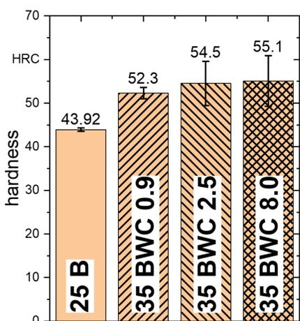
Figure 4: achieved hardness in global in-situ alloying with different WC particle sizes
