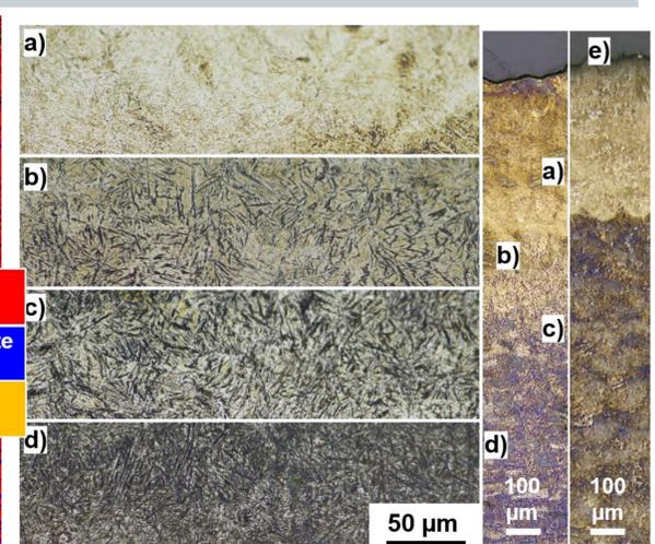
Figure 1: Overview of in-situ alloyed layer sandwiched by Bainidur with resulting hardness; sample was etched with Nital.
