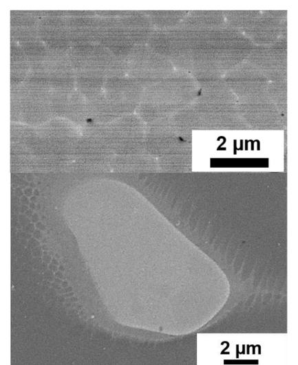
Figure 5: REM with AsB detector revealing homogenous distribution of W at grain boundaries / interdendritic phase (top) and distinct diffusion zone around remaining WC particle cores (bottom)
