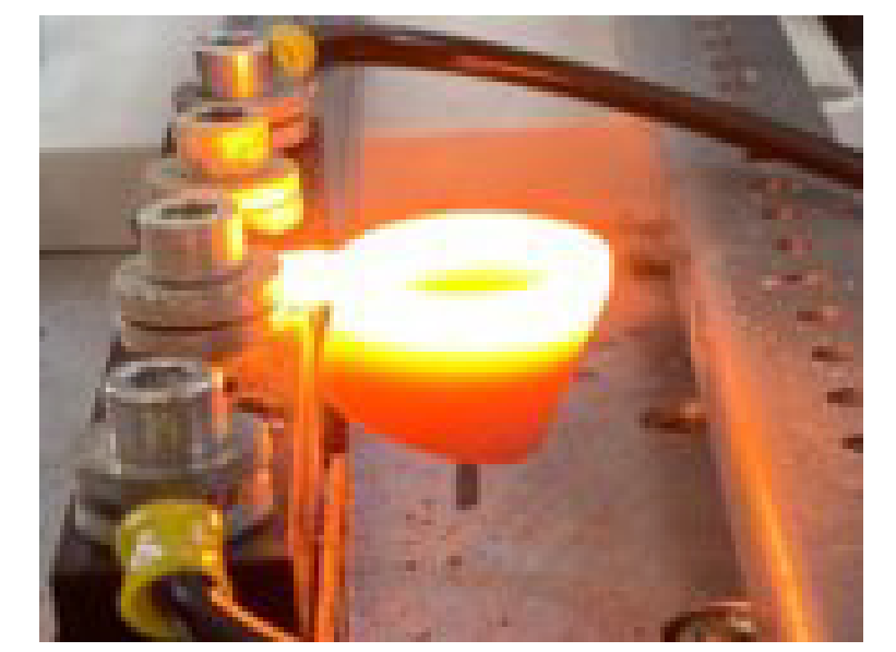
Ceramic heating element, CerAM FFF, \text{Si}_3\text{N}_4\text{-MoSi}_2 .
