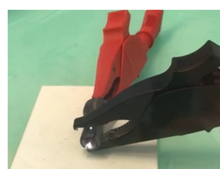
Ceramic igniter for space applications, CerAM MMJ of electrically conductive and insulating \text{Si}_3\text{N}_4\text{-MoSi}_2 .
