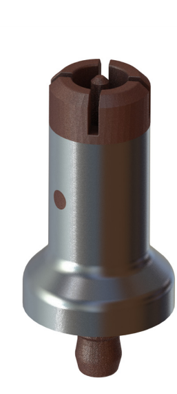
Ceramic igniter for space applications, CerAM MMJ of electrically conductive and insulating \text{Si}_3\text{N}_4\text{-MoSi}_2 .
