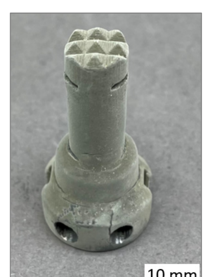
Ceramic forming tool with integrated heater, CerAM MMJ of electrically conductive and insulating \text{Si}_3\text{N}_4\text{-MoSi}_2 .
