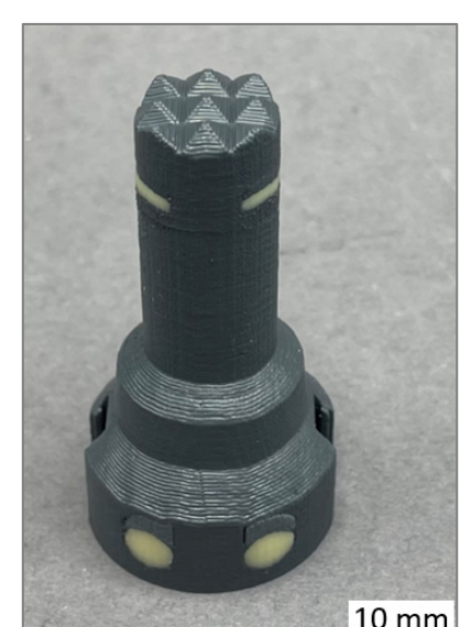
Ceramic forming tool with integrated heater, CerAM MMJ of electrically conductive and insulating \text{Si}_3\text{N}_4\text{-MoSi}_2 .
