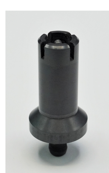
Ceramic igniter for space applications, CerAM MMJ of electrically conductive and insulating \text{Si}_3\text{N}_4\text{-MoSi}_2 .
